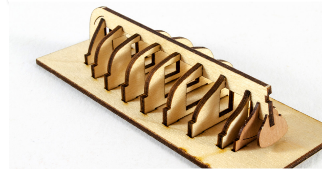
131. 18ft Cutter, optional feature : Flirt would have been fitted with a cutter like this. First, we need to build a jig for creating the hull. Cut out all parts from the 2mm MDF sheet (C1 – C11) Also cut out C14 and C15 (bulkhead and stern board) from the 1mm wood sheet. Glue parts C2 – C15 into position on the Cutter Keel C10, and lightly apply glue to a couple of these bulkheads and slot the frame/jig into the Frame Base C1.
