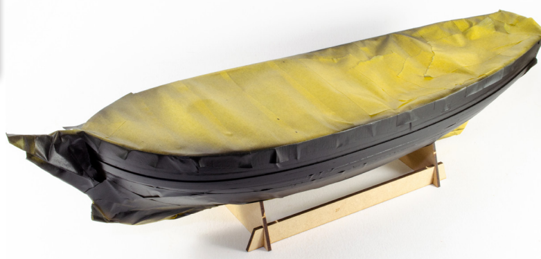
76. We will now paint the wales. You can do this in any manner you wish, but for the prototype, the whole model was masked off except for the wales, and 'Plastikote' Black was sprayed over that area in thin coats until a solid colour was achieved.
