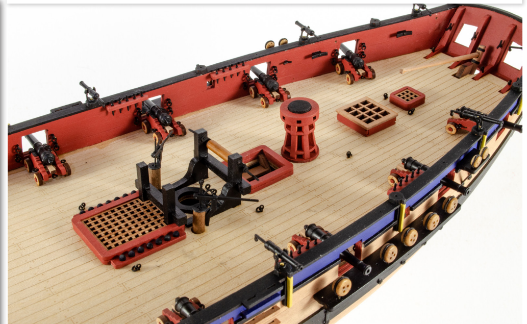
129. Now for the fun part. With a spot of glue on the underside of each wheel, glue the cannon into position, a millimetre or two away from the bulwarks. The gun cart should also be sat perpendicular to the bulwarks, and of course, centrally in the gun ports. Also glue the swivel guns into position. You can use any of the mounting points you wish. Although there are 20 points, Flirt never had more than 12 of these occupied with a gun. The guns were designed to be removable on their mounts so they would just plug into another position. When you select the position, use a 0.8mm drill and drill a few millimetres into the bulwark. Now glue the guns into position with CA.
