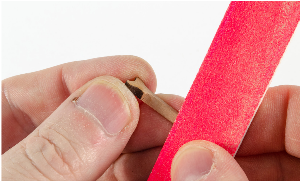
92. Remove the two Boom Crutch parts 128 from the 3mm wood sheet and bevel them as shown here.
