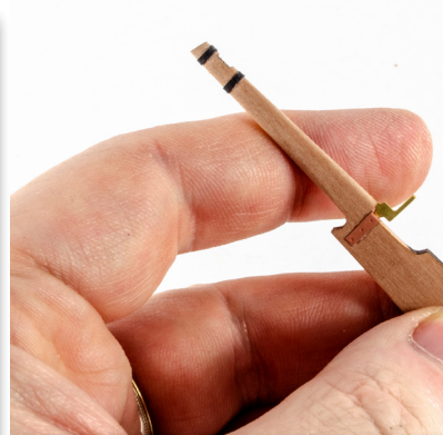
74. Cut two strips of the supplied Black Cartridge Paper F-38 (approx. 1.5mm wide) and glue to the rudder, in the positions shown.
