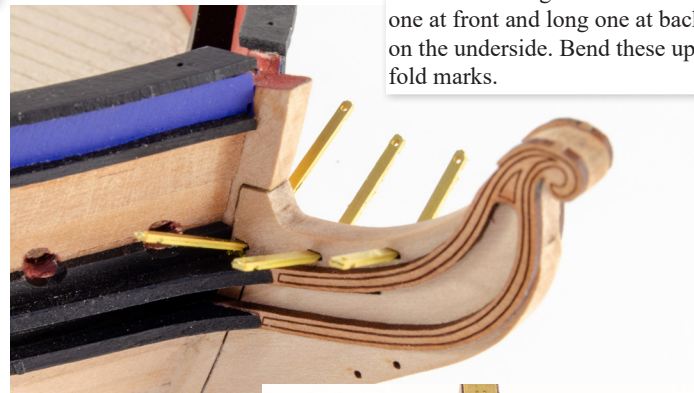
95. Remove the Bow 'V' shaped vertical rail parts (PE-37, PE-38, PE-39) from the 0.6mm PE sheet and paint the inner area in black. When dry, paint the outer area in yellow.
