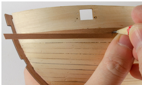
59. The second layer of planking is done in the same way as the first layer but take more care with any possible gaps. We want this layer to be as good as you can possibly make it. Now, start tapering the planks again, using a pencil to mark them as any marks can be sanded away later.
