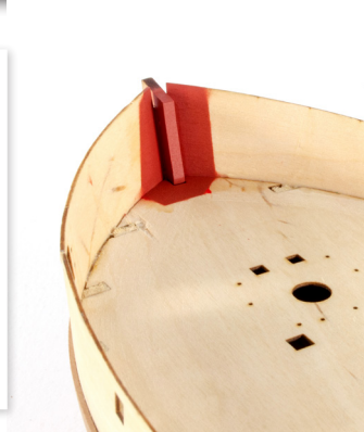
63. Before you add the laser-engraved deck, the inner bow and stern need to be painted in a suitable red colour. It will be more difficult to do this later without accidentally getting paint on the deck. For this, I used Plastikote Red Oxide primer, after first masking off the rest of the hull with adhesive tape.
