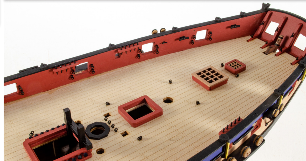
125. Glue the Main Bitt into position. This slides through the corners of the Main Hatch combing and locates into holes in the lower deck. Also fit the Aft Ladderway Combing, Skylight, and Bread Room Hatch. You can also now glue the Gratings 62 & 63 into position. Do NOT glue the grating 61 at this stage.
