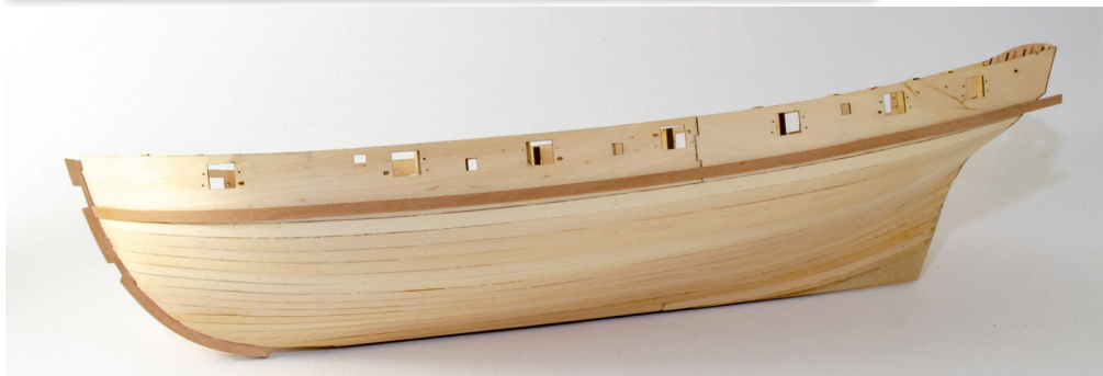
58. Take a strip of the second layer plank F-33, and cut an angle at the front, so suit the shape of the bow. Sand an inside bevel at that point so that it will push up snugly into that area without a gap. Now, this plank can be laid with either PVA wood glue or with CA gel. If you use wood glue, don't be afraid of using brass pins, as this plank will be eventually covered by the wale plank. On the prototype, I used CA gel as it gave me a good amount of time to position the plank, and a few seconds to correct any error in position. Fit the master plank to each side of the hull. Also make a small pencil mark on the Inner Stem Post which identifies the top of this master plank, for later in assembly.
