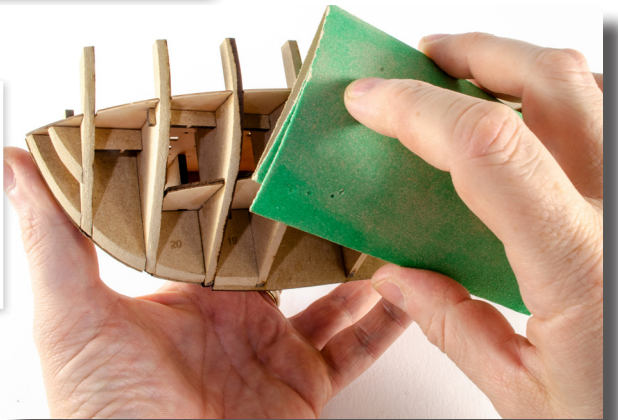
36. Before the hull can be planked, it needs to be sanded smooth. This allows the planks to run freely over the hull with maximum contact on the bulkhead edges. As we have already bevelled the bow and stern bulkheads, this task shouldn't take too long.
