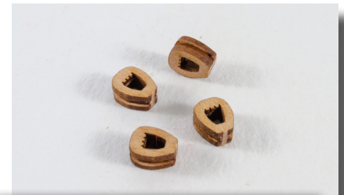
G - File away any excess material in the tab area and the blocks are ready to use
