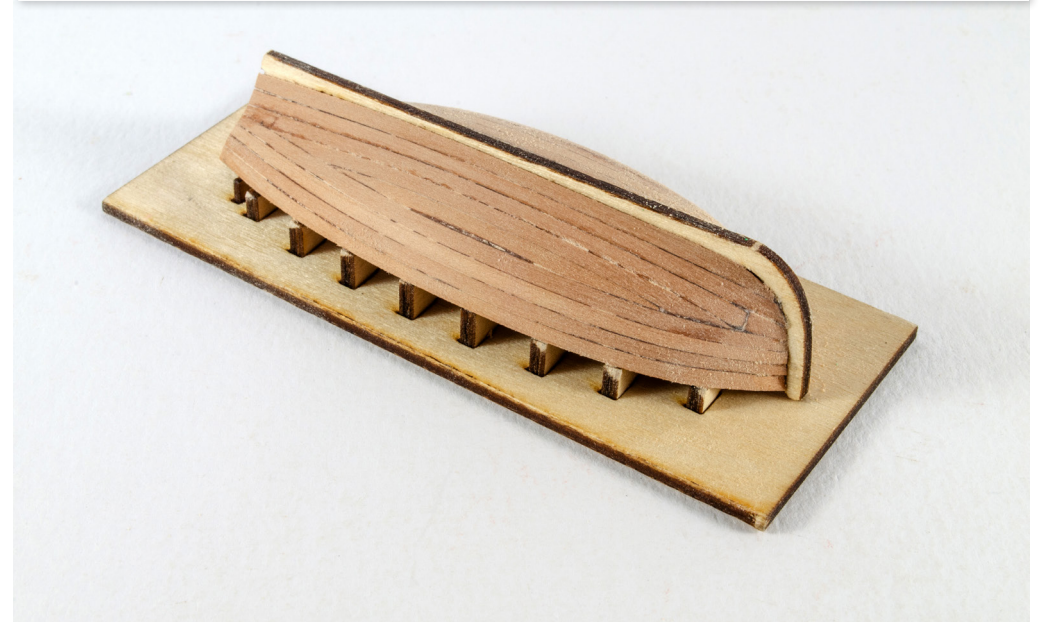
134. Run the first plank along the lip of the frames. You will need to bevel the front end of the plank to suit the bow curve. We opted to use CA gel for this as there should be no pin marks in the planks. Add additional planks and work towards the keel. Subsequent planks will need to be tapered slightly. To do this, check where the plank naturally tries to cross over the previous and make a pencil mark. From that pencil mark, cut a line towards the end of the plank, removing only about 20% of the plank width. You will need to taper and bow and stern. As you progress towards the keel and the planks don't sit easily, then let them run naturally and use small scraps of plank as stealers/infill. As a lot of the hull is painted, you won't see it.
