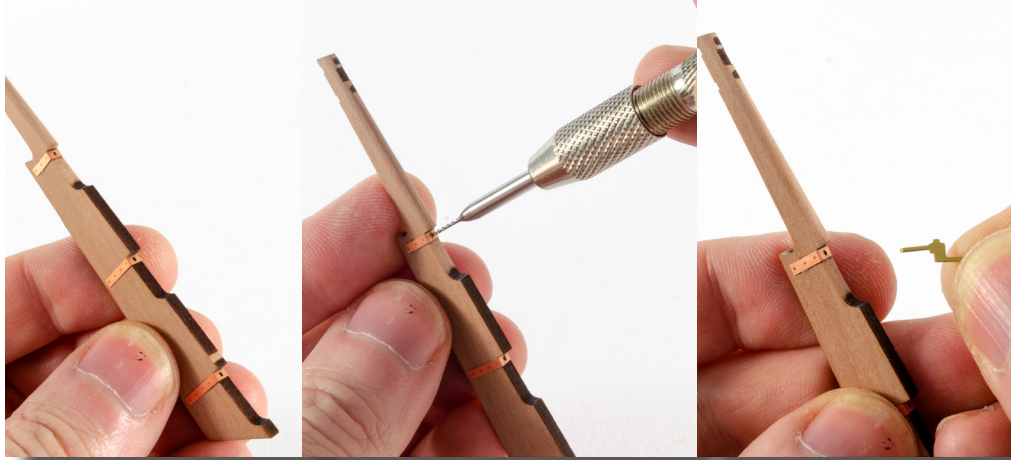
74. Cut two strips of the supplied Black Cartridge Paper F-38 (approx. 1.5mm wide) and glue to the rudder, in the positions shown.
